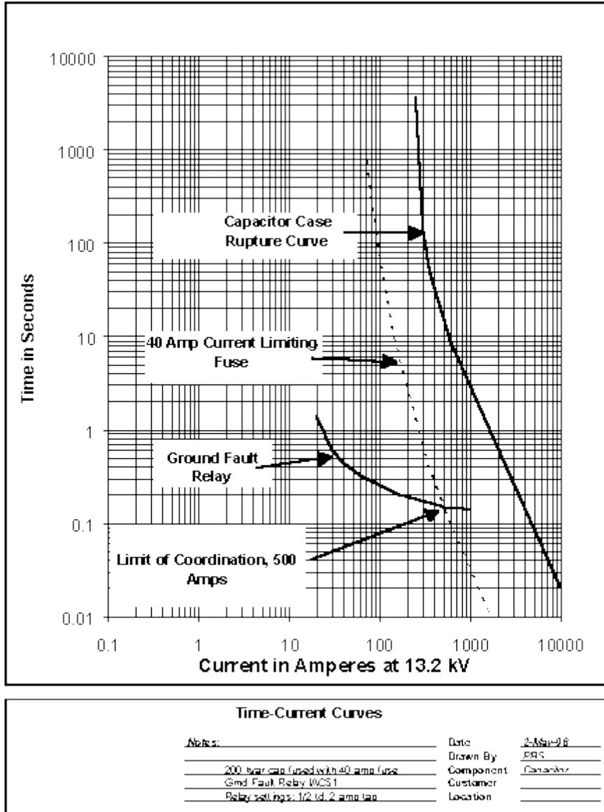
Figure 2 - Time current coordination plot of system shown in Figure 1
