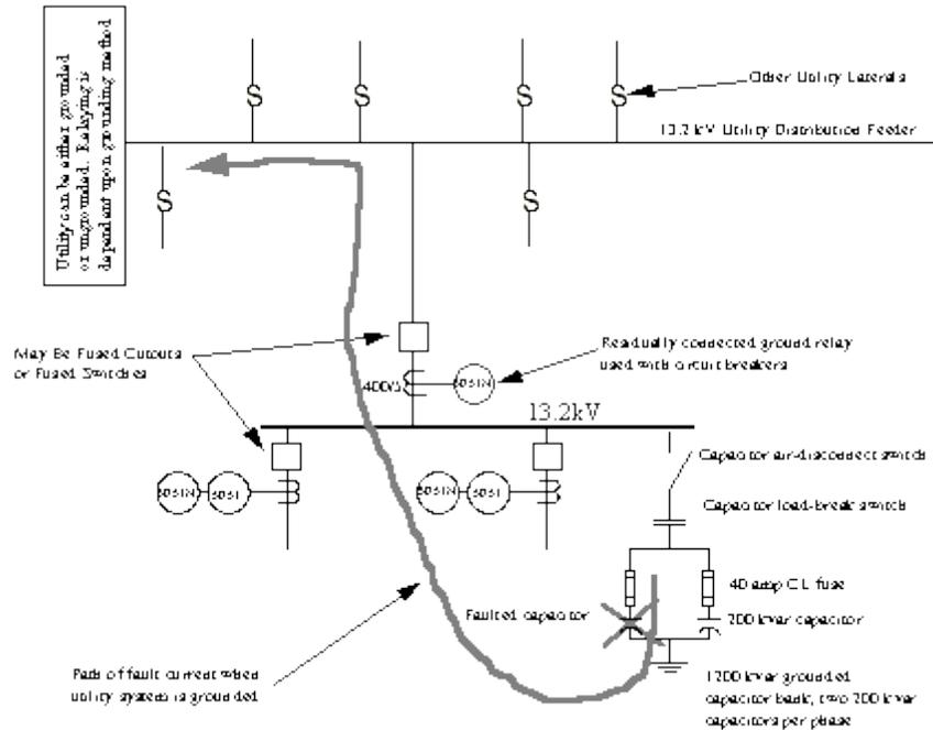
Figure 3 - Ground fault current path when industrial is connected directly to utility distribution feeder.
