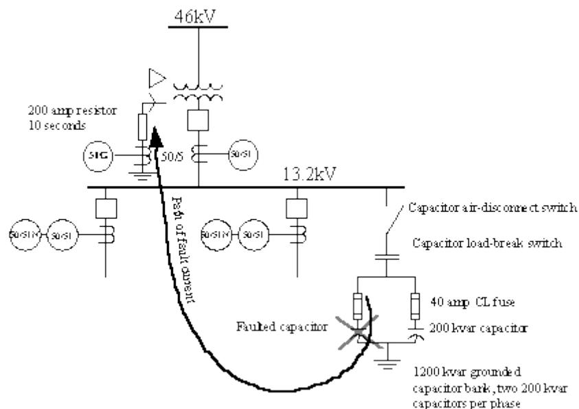
Figure 1 - Typical industrial facility showing ground fault protection system, failed capacitor, and fault current path for a failed capacitor.
